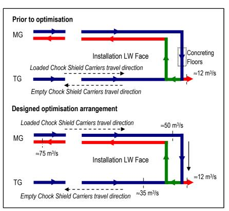
FIG 1 - Longwall panel ventilation and chock shields transport route arrangements of Mine A.
