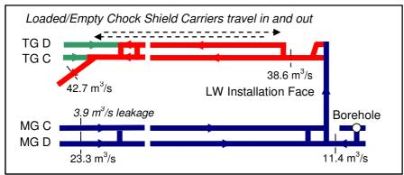
FIG 3 – Longwall panel ventilation and chock shield transport route arrangements of Mine B.
